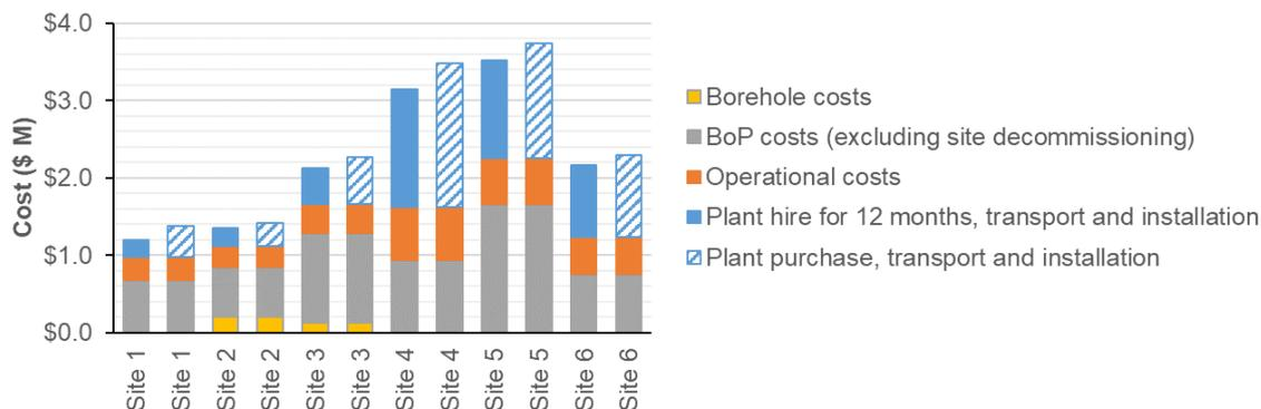
**Figure 3: Cost breakdown for the six sample sites**
