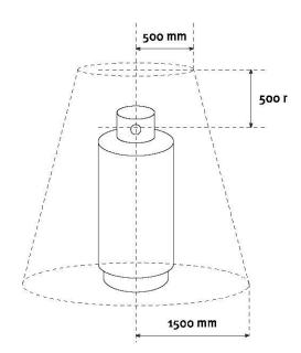
Do not use an ignition source within these distances around a gas cylinder.
