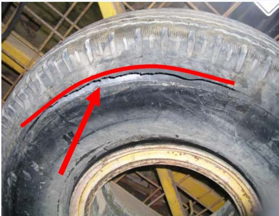
Image 6: Zipper failure on a radial tyre
