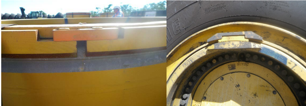
Image 8: Lock ring retainer and driver
