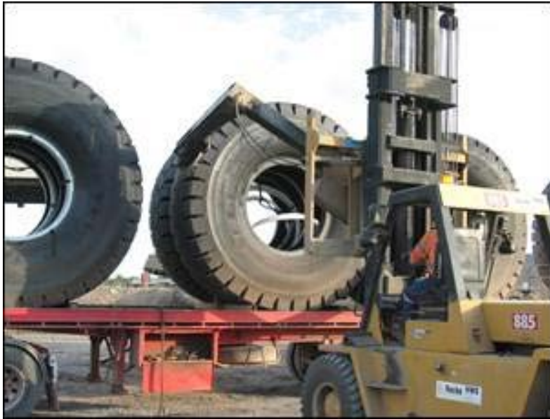
Image 4: Unloading tyre using fit-for-purpose equipment
