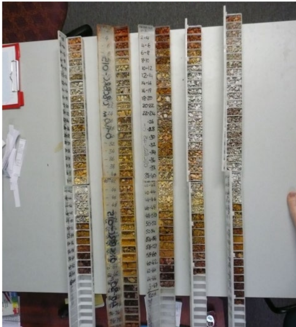
Figure 10-3. Example of preserved RC chip samples from Korella drilling in 2008.
